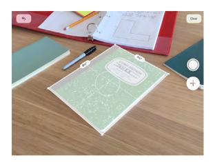
(2) Measure also detects rectangles and quickly gives you the dimension. Try identifying rectangles and having Measure automatically find the edges and the dimensions of each object.
